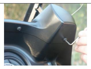
2. Install the 4 stainless steel Allen bolts in the place of the 4 bolts just removed – do not tighten; leave about ¼" thread exposed to allow the brackets to be slotted on.
