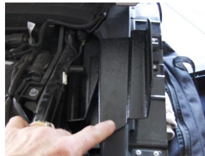
Make sure bracket is aligned with the outside edge of plastic, here.
