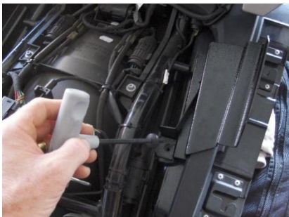
Install L&R mounting brackets Using the 2 wide flange Allen bolts
